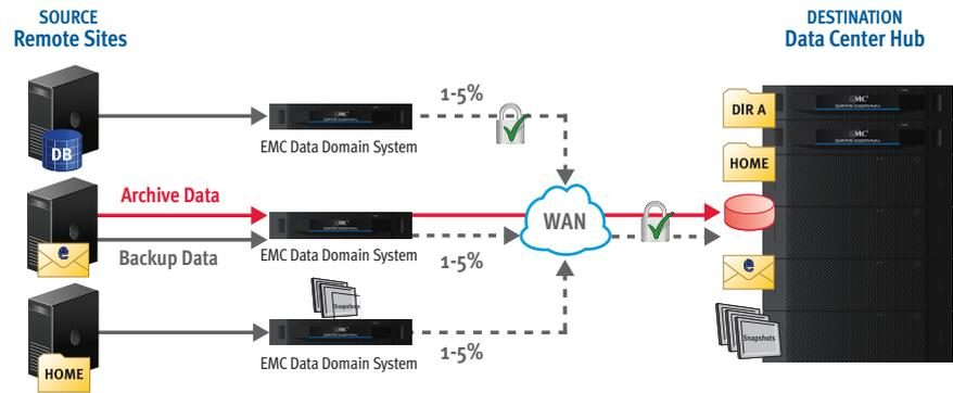
For enterprises with small datasets and 6 Mbps or less bandwidth networks, DD Replicator can further reduce the amount of data to be sent by using a low bandwidth optimization mode. This mode uses a delta compression technique to further compress the deduplicated data and eliminate redundant data within segments before sending it over the WAN. This enables remote sites with limited bandwidth to replicate and protect more of their data over existing networks.
